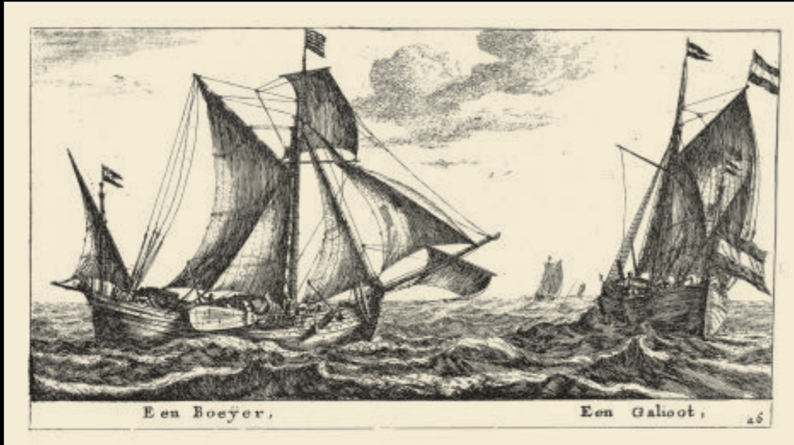
A Boeyer and a Galliot , etching by Reinier Nooms (1623-1664). Nooms placed both vessels on one plate in order to better emphasize their differences. A galliot had higher and rounder bows than a boeyer – a type of sloop – and the mast was a third of the way along its length. They were perfectly seaworthy and, fitted later with a standard three-master rigging, they continued in service until the second half of the nineteenth century.
